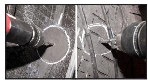
Damaged rubber and steel should be removed from the injury using a carbide cutter on a low speed air/electric drill, maximum 1,200 RPM. Drill the injury from the inside of the tire 3 to 5 times. Repeat this process from the outside.
