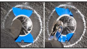
Press down the repair with your thumb from the center out. Stitch repair unit down from the center out. Remove blue poly from under cap and continue stitching toward the edge of the repair.
