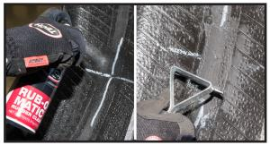
Pre-clean the inner liner 2 to 3 times with Rub-O-Matic Rubber Cleaner #704 or #704A and a scraper to remove contaminants.
