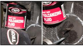
Using a spiral cement tool in a clockwise direction, apply Chemical Vulcanizing Fluid #760 to the injury 3 – 5 times. Apply a thin, even coat to the buffed surface and allow to dry 3 - 5 minutes. Additional time may be required in cold or humid conditions.
