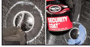
Remove the clear poly from the repair. Seal the edge of the repair unit and the over buffed area with TECH Security Coat #738 or Butyl Liner Repair Sealer #739.
