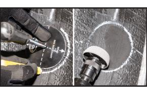
Outline the area to be buffed. Buff the outlined area with a low RPM buffer (Max 5,000 RPM) and appropriate inner liner wheel.
