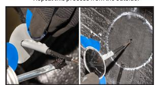
7. Apply a small amount of vulcanizing fluid to the black tapered portion of the stem. Insert the lead wire through the injury from the inside of the tire.
