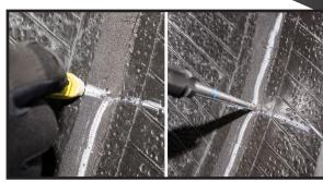
Remove the tire from the wheel. Inspect the tire for damage and defects that would make the tire non-repairable. Locate and mark all damage on the inside and outside of the tire. Insert a spiral cement tool or a probe into the injury from the inside of the tire to determine the size and angle of the injury.
