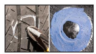
With the stem relaxed, cut off the excess stem 1/8" (3mm) above the tread surface. The tire is ready to be returned to service.
