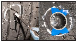
Grasp the wire with pliers on the outside of the tire and pull the stem through the tire until the cap forms a slight indentation.
