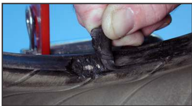
7. Deformed bead, exposed fabric or steel
