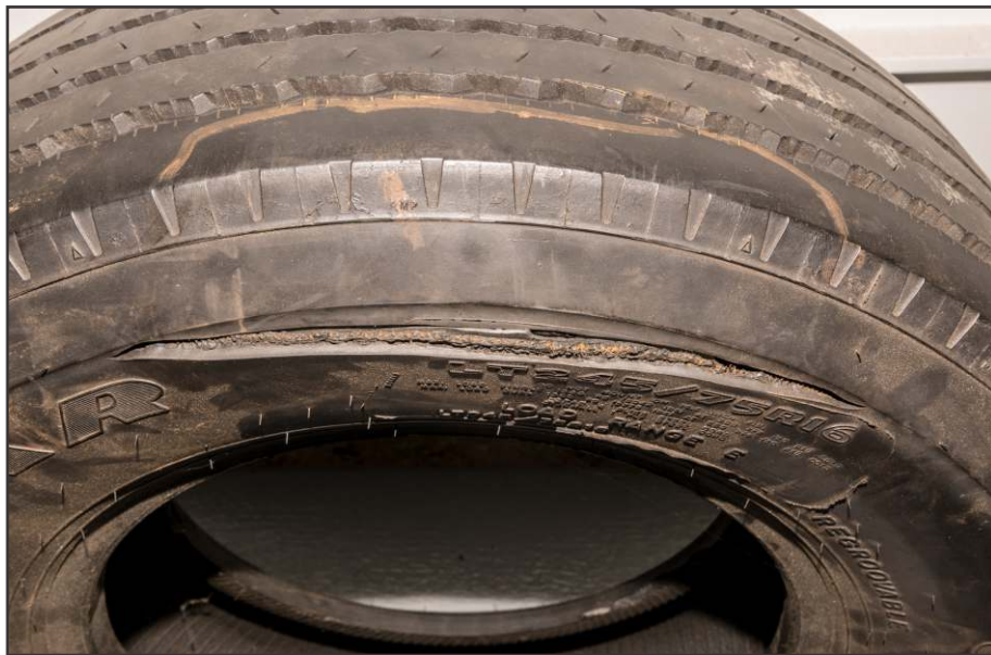
Zipper Rupture in a Light Truck Tire with steel body plies.
