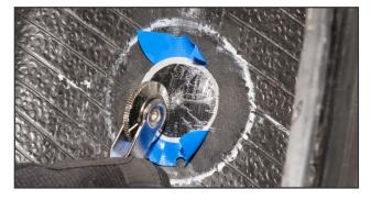
**17.** With the blue poly still positioned under the cap, stitch the repair unit from the center out using firm pressure.
