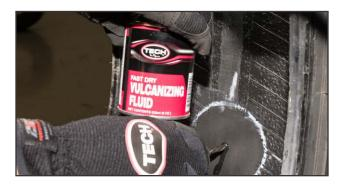
**9.** Using a fluted cement tool for injuries 6mm (1/4") or smaller or a spiral cement tool for larger punctures, apply Chemical Vulcanizing Fluid #760 or Heavy Duty Blue Vulcanizing Fluid #775 to the injury 3 to 5 times.
