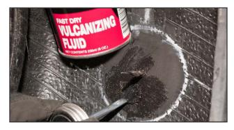
**10.** Apply a thin, even coat of Chemical Vulcanizing Fluid #760 or Heavy Duty Blue Vulcanizing Fluid #775 to the buffed surface.
