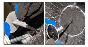
**14.** Apply a small amount of vulcanizing fluid to the black tapered portion of the stem. Relax the beads of the tire. Insert the lead wire through the injury.
