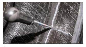
**2.** Determine the size and angle of the injury using the TRT105 injury measuring tool. If the angle exceeds 35 degrees, a two-piece repair must be used.
