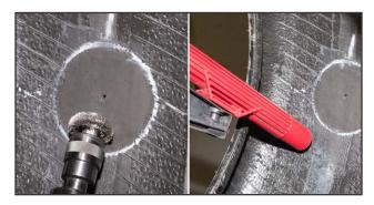
**8.** Use a soft wire brush on a low rpm buffer to remove buffing debris. Do not apply excess pressure as this could alter the buffed texture and reduce repair adhesion. Remove all debris from the tire using a vacuum, being careful not to contact and contaminate the buffed surface.
