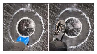
**18.** Remove the poly from the cap, press down the sides and continue stitching toward the edges of the repair. Stitch with firm pressure in the opposite direction to ensure air is removed.
