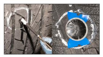
**15.** Grasp the wire with pliers and pull the stem through the tire until the cap forms a slight indentation.
