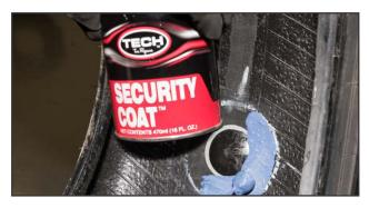
**20.** Seal the edge of the repair and the over buffed area of the inner liner with Tech Security Coat #738 or Butyl Liner Repair Sealer #739.
