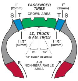
Uni-Seal Ultra repairs are designed for use in the Crown (T-T) area of the tire only.
