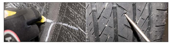
**1.** Locate and mark all damage on the inside and outside of the tire while checking for separation.
