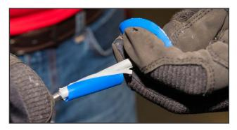
**12.** Remove the blue poly from the stem by pulling and twisting the repair as shown.
