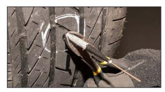
**21.** With the stem relaxed, cut off the excess 1/8" (3mm) above the tread surface.
