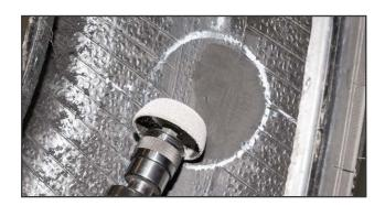
**5.** Using a low speed buffer (maximum 5,000 rpm) and an appropriate inner liner buffing wheel, buff the entire outlined area to a #1 or #2 buffed texture.
