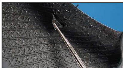
10. Tire damage from impacts
