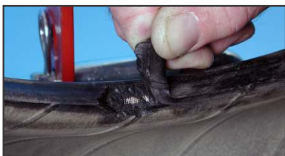
7. Deformed bead, exposed fabric or steel
