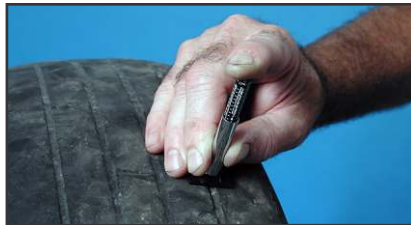
5. Excessive tread wear
