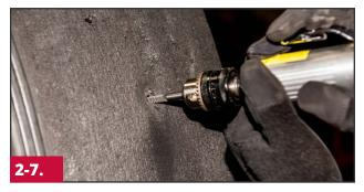
Use a carbide router on a high speed grinder (20,000 RPM min.) to remove all damaged steel and separations. Steel body cables and belts must be cut back to solid rubber. Do not use an aluminum oxide stone for this process, as they tend to scorch rubber.
