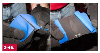
Break the perforation in the poly and peel back the poly approximately half way to expose the center of the repair unit's cushion gum. Use the poly to grasp the repair unit and keep the cushion gum clean.
