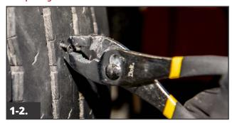
If present, remove the penetrating object. Note the angle of the injury as you remove the object.
