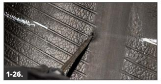
Inspect below the inner liner for splits leading away from the puncture using a #919 probe. If splits are detected, attempt to remove the additional damage with a larger carbide cutter. If the area is less than 3/8" (10mm) after the damage is completely removed, proceed to the next step. If not, treat the injury as a section repair.
