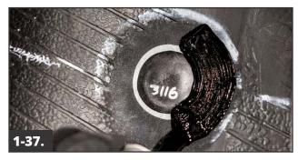
Apply Butyl Liner Repair Sealer #739 to the edge of the repair and any buffed surface outside the repair's edge.
