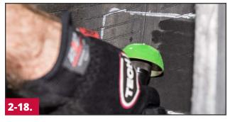
Using a fine grit buffing wheel (#RH107 or #FCRT3CR50 or equivalent) on a low RPM buffer (5,000 RPM Max.), buff the inner liner area marked to a #1 or #2 buffed texture, being careful to stay within the marked area.
