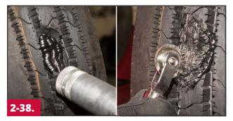
Finish filling the cavity with rope rubber until the rubber is built up 1/8" (3mm) above the tire's surface. Stitch the rubber using firm pressure to remove trapped air. The tire is now ready for curing. Refer to page 34 for instructions on how to calculate cure times.
