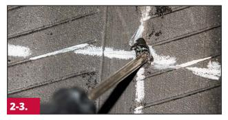
Inspect the injury with a #919 probe to determine the size and angle of the injury. Also, check for any additional damage such as looseness or impact breaks. Always look for rusted wires when the tire has steel belts or steel body plies.
