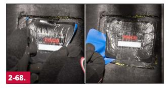
Center the repair unit over the injury, within the area where the inner liner is removed, and check for proper alignment of the bead arrows toward the tire's beads. Press down the repair unit with your thumb and stitch the repair unit from the center out using firm pressure.
