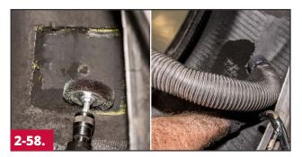
Use a soft wire brush moving from right to left to remove buffing dust and debris from the buffed area. Use a vacuum to remove this material from the tire.
