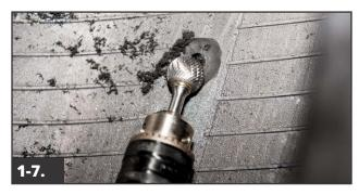
Using a small ball rasp, remove a small area of the inner liner around the injury to inspect the casing. If splits in the rubber and/or loose cables are detected, the damage must be removed. This can be accomplished by using a larger carbide cutter. If the damage is still within puncture limitations, then proceed to the next step. If not, then proceed to the Crown Section Repair procedures on page 10 of this manual.
