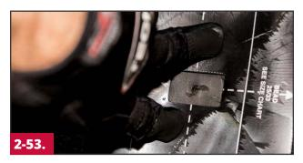
Use the appropriate size repair template and a tire crayon to mark the area where the inner liner is to be removed. If a template is not available, mark an area at least  $\frac{1}{2}$ " (13mm) larger than the repair unit being installed.
