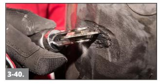
Use a Skive packing tool (#985 or #986) or a stitcher to pack the rubber into the injury channel and to remove trapped air.
