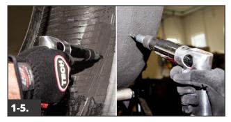
Damaged rubber and steel should be removed from the injury using a carbide cutter on a low speed air or electric drill (1,200 RPM max.). Following the angle of the injury, drill the injury from the inside of the tire 3 to 5 times. The injury should then be drilled 3 to 5 times from the outside of the tire to ensure complete damage removal.
