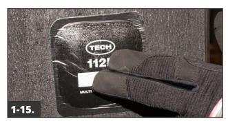
Preheat the extruder. Place a repair unit or a piece of poly over the hole on the outside of the tire. Hold firm pressure against the tire so that no air will be trapped.
