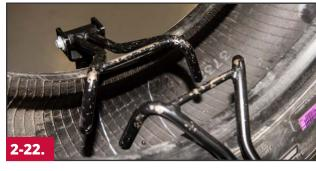
Once the cement is dry, release the spreader so that the tire is in a relaxed position. This will reduce the risk of bridging the repair unit.
