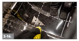
Mark the buffing area on the inner liner by placing the appropriate repair template over the injury and tracing around it with a tire crayon. Another method is to place the repair unit over the injury and mark an area  $\frac{1}{2}$ " (13mm) larger than the repair unit for buffing.
