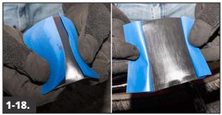
Bend the repair unit back and push up on the edges of the repair with your fingers to break the perforation on the protective poly on the back of the repair. Partially remove the poly, exposing only the middle portion of the repair unit.
