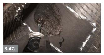
Apply a thin, even coat of cement by stippling the cement onto the inner liner. Cement the tire by applying a thin, even coat of cement by stippling the cement onto the inner liner. Use Chemical Vulcanizing Fluid #760 or Heavy Duty Blue Vulcanizing Fluid #775 for cold, or chemical cure applications. Allow the cement to dry thoroughly.
