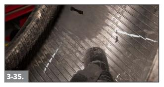
Vacuum all of the buffing dust from the tire. Do not touch the buffed surface with the vacuum as this could lead to contamination.
