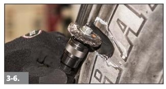
Using an encapsulated brush on a low RPM buffer, remove the remaining rubber and lightly expose only the body cables believed to be damaged, the full length of the injury. Avoid putting excess pressure on the steel cables as this could lead to additional body ply damage.
