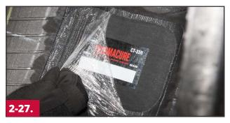
Remove the clear poly from the top of the repair unit and inspect the repair unit for trapped air. If trapped air is found, stitch the repair unit again. If the trapped air cannot be removed, remove and install a new repair unit.
