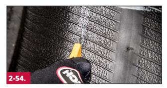
Use a sharp knife #807 to cut the inner liner along the outer perimeter of the outlined area. Lift the edge of the inner liner with the knife or a probe to determine the thickness of the material to be removed.
