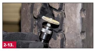
If the tread has not been buffed off, buff the outside surface of the tire 1" (25mm) wider than the skive being prepared.
