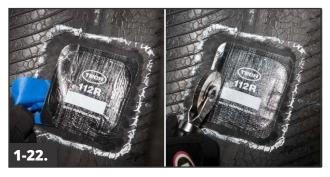
Remove the poly from under the repair unit and continue stitching from the center out, using firm pressure.
