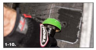
Using an RH107 or equivalent buffing wheel on a low speed buffer (max. 5,000 RPM) buff the marked area on the inner liner to a #2 buffed texture.
