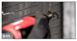
Remove any scorched rubber using a skive brush on a low RPM buffer.
