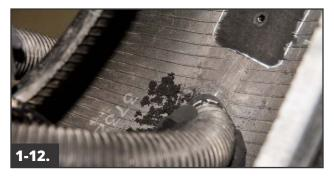
Vacuum all buffing dust from the tire. Do not touch the buffed surface with the vacuum, as this could lead to contamination.
