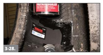
Apply Butyl Liner Repair Sealer #739 or Security Coat #738 to the edge of the repair unit as well as any buffed surface beyond the edge of the repair unit.
