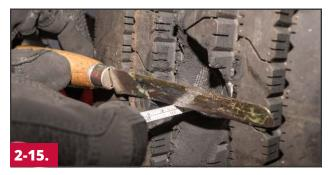
Measure the total thickness of the tire to help determine the cure time.
