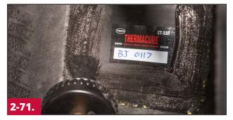
Apply a thin, even coat of Temvulc Black Cement to the outer 1" (25mm) edge of the repair unit and the buffed perimeter of the inner liner. Allow 8-10 minutes to dry.
