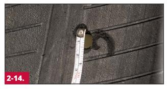
Measure the length and width of the injury at the widest opening of exposed cord to determine the proper repair unit to be used.
