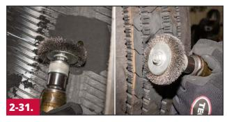
Clean the buffed area on both inside and outside of the tire using a soft wire brush on a low RPM buffer. Remove the buffing dust by lightly brushing the buffed area from the right side to the left. Repeat the process a minimum of 2 - 3times to ensure that all buffing dust is removed.
