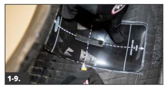
If the injury is in the outer 1.5" (40mm) of the tread, process the injury as a Reinforced Shoulder Repair. Select the appropriate size template. Position the template over the injury so the template is shifted toward the bead, keeping the injury within the template window. This will ensure that the fabric reinforcement in the repair unit extends beyond the high flex area of the tire.
