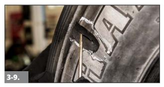
Using a probe, check to make sure that all separation has been removed.
