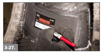
Mark the date and retread plant DOT code (if applicable) onto the repair unit with a dark or silver ink pen.
