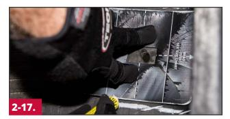
Center the appropriate repair template and use a tire crayon to mark the area on the inner liner for buffing. If a template is not available, center the repair unit over the injury and mark an area approximately  $\frac{1}{2}$ " (13mm) larger than the repair unit.
