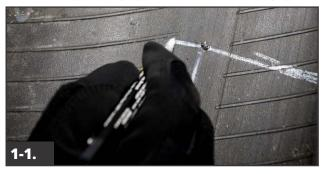
Locate and mark the damage on the inside and outside of the tire.
