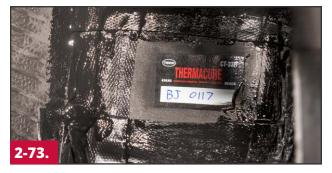
Apply Butyl Liner Repair Sealer #739 or Security Coat #738 to the Vul-Gum and the over buffed area on the inner liner.
