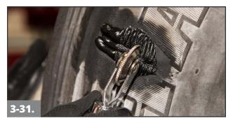
Finish filling the cavity with the extruder and stitch the rope rubber. The fill rubber should be built up to 1/8" (3mm) above the tire's outer surface. The tire is now ready for curing.
