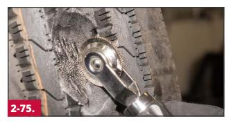
Use a skive packing tool #985 or #986 or a stitcher to pack the rubber into the injury channel and to remove trapped air.
