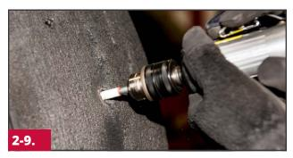
Use an aluminum oxide stone on a high speed grinder to dress any frayed steel cables into solid rubber.
