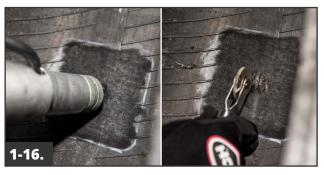
Fill the hole from the inside of the tire with LRRP rope rubber until there is a small amount of rubber above the inner liner. If a non-reinforced repair unit is used, a small amount of overfill is necessary to prevent the appearance of dimpling in the repair unit after curing. Stitch the rubber into place with a stitcher. If too much rubber remains, use a flexible knife to remove the excess rubber to avoid trapping air under the repair unit, then stitch the rubber again.
