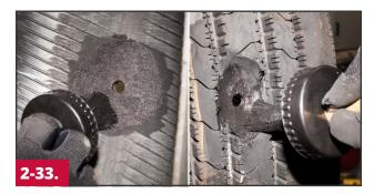
Apply a thin, even coat of Temvulc Black Cement #1082 to the buffed surfaces on both the inner liner and the outside skive. Allow to dry 8-10 minutes. More drying time may be necessary in cold and/or humid conditions.
