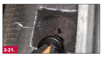
Apply a thin, even coat of cement by stippling the cement onto the inner liner. Use Chemical Vulcanizing Fluid #760 or Heavy Duty Blue Vulcanizing Fluid #775 for cold, or chemical cure applications. Use Temvulc Black Cement #1082 for heat cure applications such as retreading. Allow the cement to dry thoroughly.
