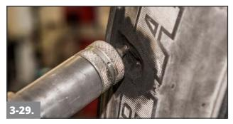
Using a preheated extruder, apply rope rubber into the cavity while exerting firm pressure with the extruder to prevent trapping air.
