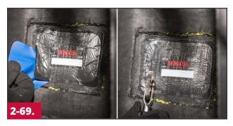
Remove the remaining poly from under the repair unit, press the repair unit down and continue stitching form the center out, toward the edges of the repair unit.
