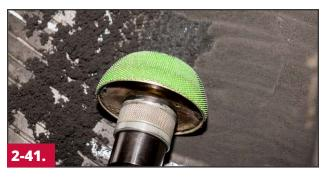
Using a fine grit buffing wheel (#RH107 or #FCRT3CR50 or equivalent) on a low RPM buffer (5,000 RPM max.), buff the inner liner area marked to a #1 or #2 buffed texture, being careful to stay within the marked area.
