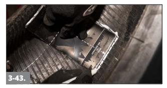
Use the appropriate size template and a tire marker to mark an area on the inner liner for buffing. When placing the template be sure to place the lines for the reinforcement package outside of the flex area of the tire.
