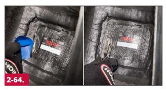
Remove the remaining poly from under the repair unit, press the repair unit down and continue stitching the repair unit toward the edges.
