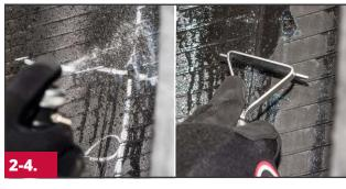
Place the tire so the repair area is at the 7-9 o'clock position to allow solvent and buffing dust to fall to the bottom of the tire. Pour or spray Rub-O-Matic #704 or 704A or Citrus Based Rubber Cleaner #705C on the inner liner and use a #933 scraper to clean the inner liner. Repeat this process 2-3 times to remove any foreign materials that might contaminate the repair area or buffing tools.
