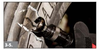
Use a knife or rotary gouge on a low RPM buffer (5,000 RPM max.) to remove all loose or damaged rubber. Be careful to avoid contacting the steel cables as this could lead to additional damage.
