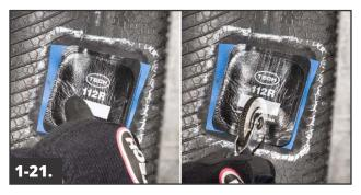
Press down the center of the repair unit with your thumb. Begin stitching from the center outward, using firm pressure. Stitch out to the folded poly.
