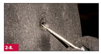
Using a probe, check to make sure that all separation has been removed.
