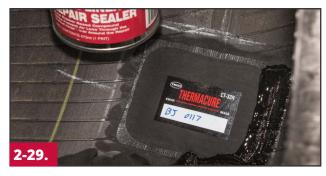
Apply Butyl Liner Repair Sealer #739 or Security Coat #738 to the edge of the repair unit as well as to any buffed surface not covered by the repair unit.
