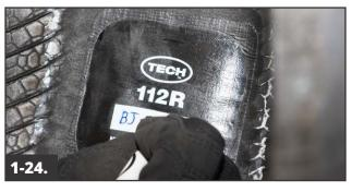
Initial and date the repair unit with a tire marker or silver inkpen for proper tracking.
