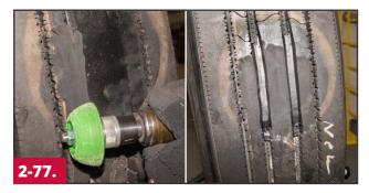
After the tire is cured, inspect the repair unit and fill rubber for proper cure. Buff any excess fill material flush with the tread surface. If necessary, use a regroover to cut any filled-in grooves back into the tread. The tire can now be returned to service.
