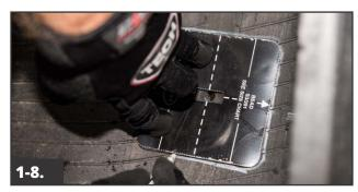
Select the correct repair unit to be installed. Center the proper repair unit template over the injury and use a tire marker to outline the template for buffing. It is also acceptable to use the repair unit and mark an area at least  $\frac{1}{2}$ " (13mm) larger than the repair unit for buffing.
