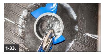
Press down the repair with your thumb, working from the center out. With the poly still in place under the cap, stitch the repair from the center out using firm pressure.
