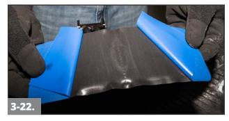
Break the perforation in the blue poly on the back of the repair unit. Peel the poly back on both sides to expose the center of the repair unit's cushion gum, while leaving the edges covered. Use the poly to grasp the repair unit and prevent contamination of the cushion gum.
