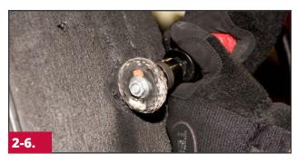
Use an encapsulated wire brush on a low RPM tool to remove any remaining rubber and to expose damaged cords. Be careful not to expose too much steel. This could lead to reduced adhesion of the fill material to the tire.
