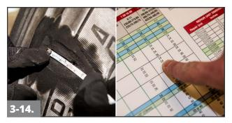
Measure the width and length of the injury at the widest opening of removed body ply. Use these measurements to select the proper repair unit from the Centech & Thermacure Radial Repair Chart (#CT).
