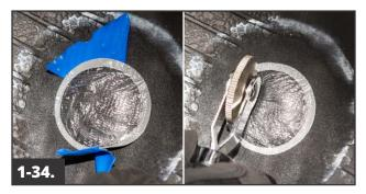
Remove the remaining poly from under the repair unit. Press down the repair and stitch firmly in multiple directions from the center out to ensure all air is removed.
