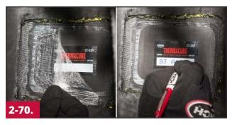
Remove the protective poly from the top of the repair unit. Mark the date and retread plant DOT code (if applicable) onto the repair unit using a dark or silver pen.
