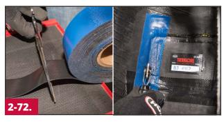
Cut four strips of 2" (50mm) wide Vul-Gum cushion gum #864 that are approximately 2" (50mm) longer than each side of the repair unit. Place each strip of rubber overlapping the edges of the repair unit and the inner liner and stitch. Make sure the gum covers both the edge of the repair unit and the buffed area on the inner liner to ensure that it properly contains the sealant material under the inner liner.
