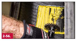
Using a twisted wire brush on a low RPM buffer, lightly buff the remaining sealant material from the exposed area. Make sure to completely remove the sealant material from the edges and corners where the inner liner has been cut away.
