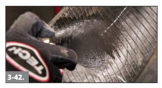
After the tire is cured and has cooled to room temperature, pour or spray Rub-O-Matic #704 or 704A or Citrus Based Rubber Cleaner #705C on the inner liner and use a #933 scraper to clean the inner liner. Repeat this process 2-3 times to remove any foreign materials that might contaminate the repair area or buffing tools.
