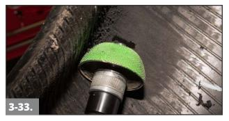
Using a fine grit buffing wheel (#RH107 or #FCRT3CR50 or equivalent) on a low RPM buffer (5,000 RPM max.), buff an area approximately 1  $\frac{1}{2}$ " (40mm) in all directions around the injury.
