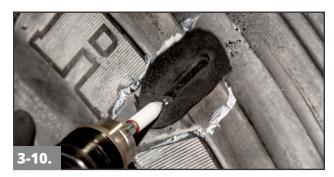
Use an aluminum oxide stone on a high RPM buffer to dress any frayed steel cables into solid rubber. Aluminum oxide stones are only used to finish dressing steel, not for cutting through steel cables, as they tend to scorch rubber.
