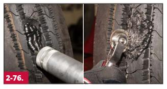
Finish filling the cavity with rope rubber until the rubber is built up 1/8" (3mm) above the tire's surface. Stitch the rubber using frim pressure to remove trapped air. The tire is now ready for curing.
