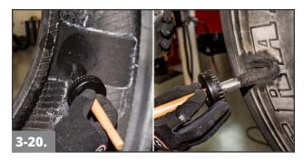
If installing a Thermacure repair, apply a thin, even coat of TemVulc black cement to the buffed inner liner and skive areas. If installing the repair unit chemically, use Chemical Vulcanizing Fluid. Cement Drying Times: TemVulc: 8-10 minutes; Chemical Vulcanizing Fluid: 3-5 minutes; Heavy Duty Blue Vulcanizing Fluid: 5-8 minutes. Additional time is necessary in cold and/or humid conditions.
