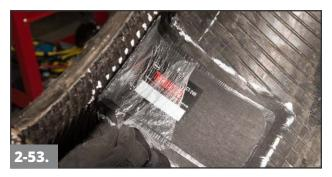
Remove the clear poly from the top of the repair unit and inspect the repair unit for trapped air. If trapped air is found, stitch the repair unit again.
