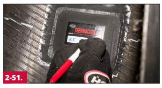
Use a dark ink pen or marker to mark the date and retread plant DOT code (if applicable) onto the repair unit.
