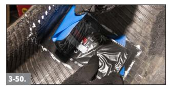
Fold and position the repair unit so that the repair unit's bead arrows are pointed toward the tire's beads. Center the repair unit over the injury and place the center of the repair unit against the inner liner. Release the repair unit and check that the repair unit is properly aligned and centered. If the repair unit is not centered, and/or straight, lift and reposition the repair unit.
