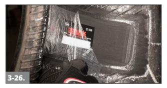
Remove the clear poly from the top of the repair unit and inspect the repair unit for trapped air. If trapped air is found, stitch the repair unit again until all air is removed. If the trapped air cannot be removed, remove and install a new repair unit.
