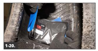
If the injury is a Reinforced Shoulder Repair, fold the repair unit, and then position the repair unit so that it is completely within the buffed area, aligning the bead arrows to the tire's beads. Release the repair unit and check the alignment. If the repair unit is not straight and/or completely within the buffed area, lift the repair unit and reposition.
