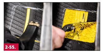
Using a tire regroover with a wide flat blade (W-5 or W-6 style) set to the appropriate depth, cut the inner liner and sealant material out of the tire in the outlined area, leaving a thin layer of the sealant on the casing. An alternative method is to completely remove the cut inner liner by pulling it out with a pair of pliers before using the regroover to remove the sealant material.
