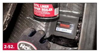
Apply Butyl Liner Repair Sealer #739 or Security Coat #738 to the edge of the repair unit as well as to any buffed surface not covered by the repair unit. Allow the tire to sit for 24 hours before returning to service.
