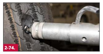
Pre-heat the extruder gun. Exerting firm pressure on the extruder, apply TRRP or LRRP rope rubber into the injury channel from the outside of the tire.
