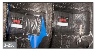
Remove the blue poly from under the repair unit and continue stitching outward using firm pressure.
