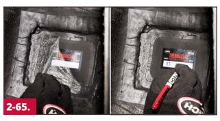
Remove the protective poly from the top of the repair unit. Mark the date and retread plant DOT number (if applicable) onto the repair unit using a dark or silver pen.
