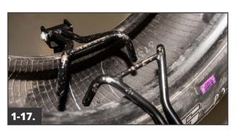
Release the spreader so the tire is in a relaxed position before installation of the repair unit.
