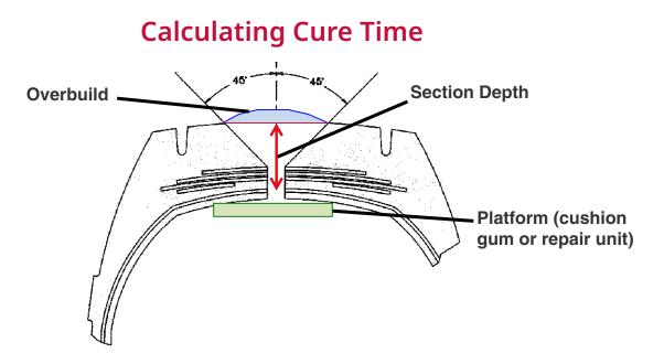
To determine the cure time measure the section depth (thickness of the tire at the deepest point of the skive). Then add this to the thickness of the repair and overbuild of the filler rubber. The total thickness is then multiplied by the cure rate of the rubber being used. **This does not include equipment warm up time.**
