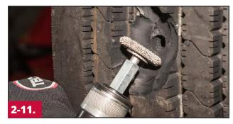
Use a medium grit rasp or encapsulated brush on a low speed buffer to buf the rubber above the steel belts. The skive should be angled at 45° and buffed to a #2 or #3 buffed texture.
