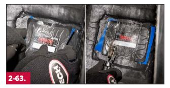
Center the repair unit within the prepared area and check for proper alignment of the bead arrows toward the tire's beads. Press down the center of the repair unit with your thumb and stitch the repair unit from the center out, using firm pressure.
