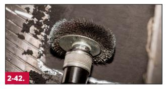
Clean the buffed area on both inside and outside of the tire using a soft wire brush (#S892) on a low RPM buffer. Remove the buffing dust by lightly brushing the buffed area from the right side to the left. Repeat the process a minimum of 2 - 3 times to ensure that all buffing dust is removed.
