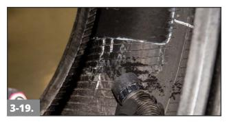
Vacuum all of the buffing dust from the tire. To avoid contamination, do not touch the buffed surface with the vacuum.
