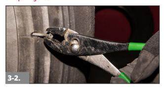
If present, remove the penetrating object. Observe the angle of the injury as you remove the object.
