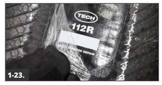
Remove the clear poly from the top of the repair unit and inspect the repair unit for trapped air. If trapped air is found, stitch the repair unit again until all trapped air is removed. If the trapped air cannot be removed, remove the repair unit and return to step 1-18 and install a new repair unit.
