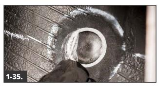
Remove the clear poly from the top of the repair unit and inspect the repair for trapped air. If trapped air is found, stitch the repair unit again until all air is removed. If the trapped air cannot be removed, remove the repair unit. Return to step 1-30 and install a new repair unit.
