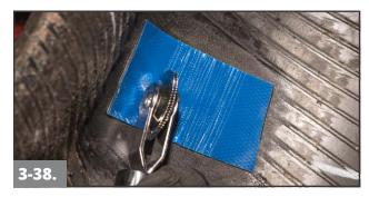
Apply the Vul-Gum to the buffed area on the inner liner. Stitch the Vul-Gum from the center out. Remove the poly from the Vul-Gum after it is thoroughly stitched.
