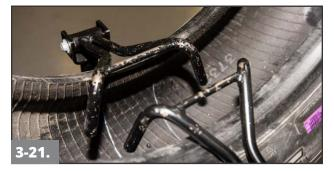
Release the spreader so that the beads of the tire are in a relaxed position prior to installing the repair unit. This will help prevent bridging of the repair unit.
