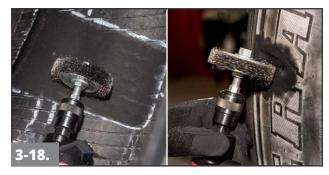
Clean the buffed surfaces on both the inside and outside of the tire using a soft wire brush on a low RPM buffer. Remove the buffing dust by lightly brushing from the right side of the buffed surface to the left side. Repeat 2-3 times or until all of the buffing dust is removed. To prevent contamination, stay within the marked area.
