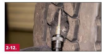
On high tread tires, the tread grooves must be buffed with a pencil rasp (#RH626 or #FCRTNR70) on a low speed buffer.
