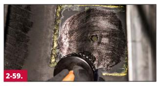
Apply a thin, even coat of Temvulc Black Cement #1082 to the entire buffed surface on both the inside and outside of the tire. Allow 8-10 minutes drying time. Additional time will be necessary in cold or humid conditions.
