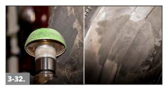
After the tire is cured and has cooled to room temperature, buff the cured rubber on the outside of the tire flush with the tire's surface. The tire can now be returned to service.
