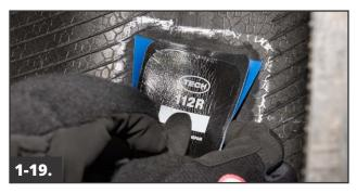
Fold the repair unit and position the repair unit, aligning the beads arrows to the tire's beads if a reinforced repair is being used. Center and place the repair unit over the injury. Release the repair unit to check for proper placement and alignment. If the repair unit is not centered and/or straight, lift the repair and reposition.
