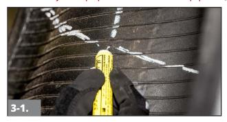
Mark the injury on both the inside and outside of the tire using a tire crayon.
