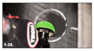
Using a fine grit buffing wheel on a low RPM air buffer (5,000 RPM max), buff the marked area on the inner liner to a #1 or #2 buffed texture, staying within the marked area.
