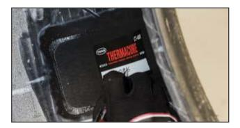
**23.** Mark the date, repair technician initials (optional), and retread plant DOT code onto the repair unit. Use a dark ink pen or marker.
