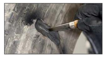
**5.** Separate damaged cables by cutting as close as possible to the damage with a sharp knife.
