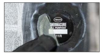
**19.** Remove the clear Mylar from the top of the repair unit by lifting from the edge of the repair and inspect the repair unit for trapped air. If trapped air is found, stitch the repair unit again. Extra attention should be paid to the repair unit edges to ensure they are thoroughly stitched.
