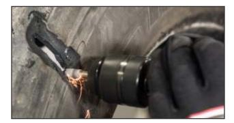
**7.** Use an aluminum oxide stone on a high RPM buffer to dress any frayed steel cables into solid rubber. Aluminum oxide stones are only used to finish dressing steel, not to cut through steel cables, as they tend to scorch rubber.
