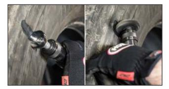
**4.** Remove all loose or damaged rubber using a knife or rotary gouge on a low RPM tool (5,000 RPM max) without damaging steel body cables. Then expose damaged cables with an encapsulated brush.
