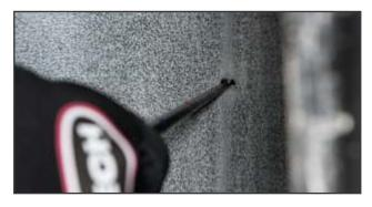
**1.** Inspect the damage with a probe to determine the size and angle of the injury. Also, check for any additional damage such as separations, looseness, or impact breaks. Always look for rusted cables when the tire has steel belts or steel body plies.
