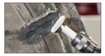
**9.** Buff the rubber above the body ply using a low RPM buffer and a medium grit rasp or encapsulated brush. Buff to an #2 or #3 buffed texture.
