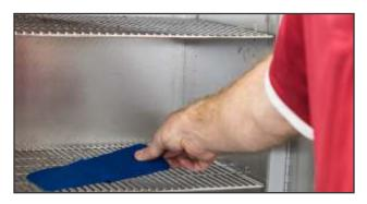
**12.** Repair units can be installed with or without floater gum. In order to achieve proper green tack, the repair unit must be heated to a temperature of between 140°F and 160°F (60°C to 72°C). 111R, 112R through CT-24R repairs should be pre-heated 5 to 7 minutes. For repairs larger than a CT-24R, the pre-heating time is 8 minutes. TECH recommends the use of an oven so that multiple repair units can be heated at the same time, saving time and money.
