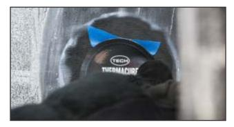
**16.** Fold the repair unit and position it, aligning the bead arrows to the tire's beads if a reinforced repair is being used. Center the repair unit over the injury. Release the repair unit and check the alignment. If the repair unit is not centered and/or straight, lift and reposition.
