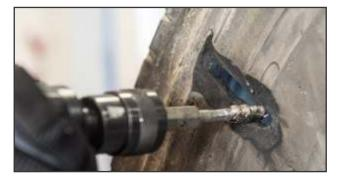
**8.** Remove any scorched or burned rubber using a soft wire skive brush on a low RPM buffer.
