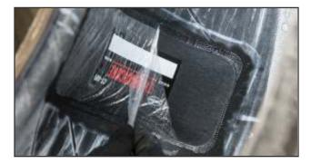
**22.** Remove the clear poly from the repair unit.
