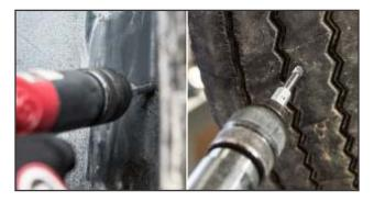
**4.** Damaged rubber and steel should be removed from the injury using the appropriate size carbide cutter on a low speed drill (maximum 1,200 rpm). Drill the injury from the inside of the tire 3 to 5 times, followed by 3 to 5 times from the outside of the tire to ensure complete damage removal.
