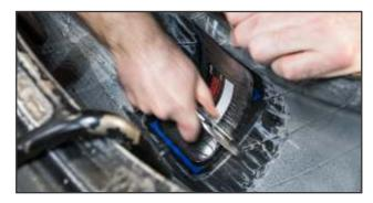
**19.** Press down the repair with the side of your hand. Stitch the repair from the center out. Again, proceed quickly so that the repair unit does not cool.
