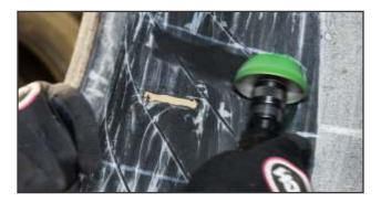
**14.** Using an approved buffing wheel on a low RPM buffer, buff the inner liner area marked to a #1or #2 buffed texture, staying inside the marked area. Be sure to completely remove all bladder patterns during this process to ensure a proper bond of the repair unit to the tire.
