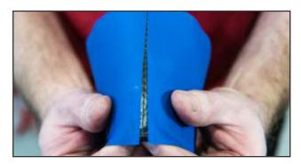
**11.** Any time that the repair is going to be heated, the slit in the poly must be broken prior to placing the repair unit in the oven so that the heated poly does not cause wrinkles in the repair gum. These wrinkles are very difficult to stitch out.
