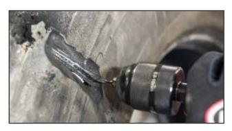
**6.** Remove all damaged steel at a 90° angle to the tire using a high RPM buffer (min. 20,000 rpm). Steel cables must be cut back into solid rubber. Inspect the area once the damage has been removed to assure that no damaged steel, splits, separations or rust remains in the tire.
