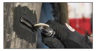
**25.** Support the repair unit on the inside of the tire. Stitch the rubber to work out any air and to assure good contact with the tire.
