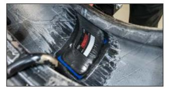
**18.** Center and align the repair using the hash marks. It is extremely critical that the alignment and centering are correct. To ensure that the repair remains warm throughout the installation it must be stitched as soon as it touches the buffed surface. If the repair unit is allowed to cool, it will not have enough green tack to properly bond to the inner liner.
