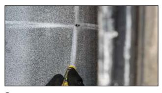
**2.** Use an approved marker to place indicating marks on the injury area. Remove the penetrating object. Observe the angle of the injury as you remove the object.
