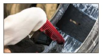
**16.** Vacuum all buffing dust from the tire. Do not touch the buffed surface with the vacuum, as this could lead to contamination. Use of an air hose to remove dust is not recommended as it will lead to contamination of the repair area.
