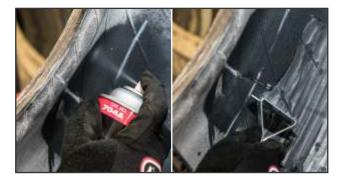
**3.** Pre-cleaning the inner liner is optional depending on the local requirements for combustible products such as 705C, Citrus Cleaner. Pre-cleaning can be accomplished using 705C Citrus Based Rubber Cleaner and a scraper 2 to 3 times to remove contaminants from the inner liner.
