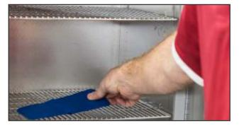
**8.** Select the correct repair unit to be installed. Refer to chart on page 11. If repairing through a mold cure process, use a reinforced repair unit such as a 112R or CT-20R. In order to achieve proper green tack, the repair unit must be heated to a temperature of between 140°F and 160°F (55°C to 72°C). For repairs such as small nail hole repairs and the CT20R this takes 5 to 7 minutes.
