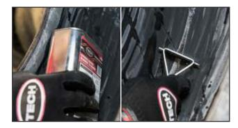
**3.** Place the tire so the repair area is in a 5 or 7 o'clock position to allow the buffing dust to fall to the bottom of the tire. Where permitted, the area can be cleaned by using a solvent free, pre-buff cleaner, such as 705C Citrus Based Rubber Cleaner, to prevent contamination of tools. Use a scraper tool to remove contaminants. Repeat this process 2 or 3 times until all contaminants have been removed from the repair area.
