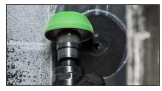
**10.** Using an approved buffing wheel on a low RPM buffer, buff the inner liner area marked to an #1 buffed texture, staying inside the marked area. Be sure to completely remove all bladder patterns during this process to ensure a proper bond of the repair unit to the tire.
