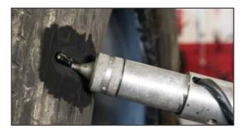
**24.** All injuries should be filled with a rubber that is approved for use without black retread cement. It is critical to apply one layer of rope rubber to the skive area due to the lack of black cement.
