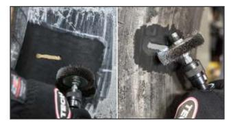
**15.** Clean the buffed areas, both on the inside and outside of the tire, using a soft wire brush on a low RPM buffer. Remove buffing dust by lightly brushing from the right side of the buffed surface to the left side. Repeat until all dust is removed.
