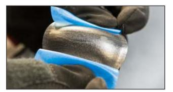
**15.** Release the spreader so that the beads are in a relaxed position before installation of the repair unit. Remove the repair unit from the oven; break the perforation in the poly and peel back the poly approximately half way to expose the center of the repair unit's cushion gum. Use the poly to grasp the repair unit and keep the cushion gum clean.
