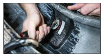
**21.** Finish stitching to the outer edge of the gum on the repair. Then stitch the repair in the opposite direction from the center out.
