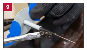
Apply a small amount of vulcanizing fluid to the black tapered portion of the repair. Push the lead wire through the prepared hole in the tire.
