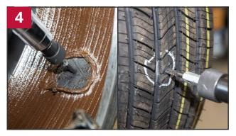
Damaged rubber and steel should be removed from the injury using a proper size carbide cutter on a low speed air/electric drill, maximum 1,200 rpm. Drill the injury from the inside of the tire 3 to 5 times, followed by 3 to 5 times from the outside.
