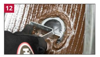
If the Sealant was scraped away from the injury, use a scraper to spread the material back over the repair unit.
