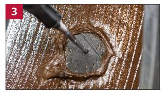
Determine the size and angle of the injury using the TRT105 injury measuring tool. If the injury exceeds  $35^{\circ}$  or  $\frac{1}{4}$ " (6mm) in size, **DO NOT** repair the tire.
