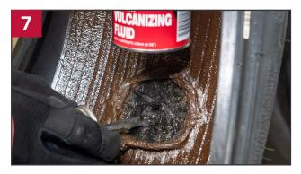
If the sealant was removed from the inner liner, apply a very thin, even coat of TECH Chemical Vulcanizing Fluid to the exposed inner liner and allow to dry for 3-5 minutes. Allow additional drying time in cold and/or humid weather conditions.
