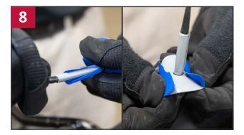
Remove the blue poly from the stem and the cap of the Uni-Seal without touching the gray cushion gum. Reposition the poly onto the cap to prevent contamination of the gray gum.
