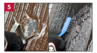
If the sealant layer is tacky, the repair can be placed directly onto the sealant, and proceed to step 8. If the Sealant has lost its tack, then scrape the sealant away from the injury, creating an area on the inner liner slightly larger than the Uni-Seal repair.
