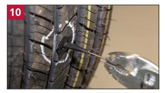
Grasp the lead wire on the outside of the tire and pull the repair with even pressure through the tire until the cap forms a slight indentation. Do not over pull.
