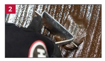
If possible, use a scraper to move the sealant material away from the injury. This will prevent contamination of the carbide cutter.
