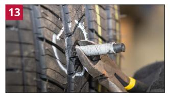
Cut the stem off on the outside of the tire approximately 1/8" (3mm) above the tread surface. If the injury is in the tread groove, the stem can be cut off flush to the tread surface. The tire is now ready to return to service.
