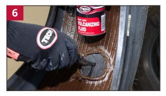
Apply TECH Chemical Vulcanizing Fluid #760 into the injury 3-5 times using a Tech #910 or #915 Cement Tool.
