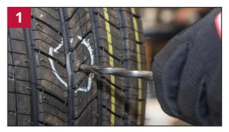
Locate and mark the injury on the outside of the tire. Insert a probe into the injury from the outside of the tire to determine the location of the injury on the inside of the tire.
