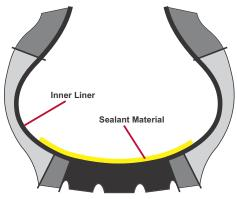
The following is a guide for proper repair of Self-Sealing passenger tires.
