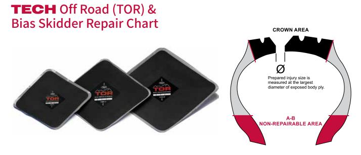
**CHART INSTRUCTIONS:** For proper repair unit selection, determine the size of the injury in the tire by measuring largest cord area removed. Locate the correct injury size along the top row of the chart. Now locate the tire's ply rating (load range) along the left column of the same chart. The repair unit number shown in the box where these intersect is the correct repair unit to use.
