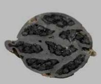
Cross Section of Multiple Permacure Repairs Vulcanized Together
