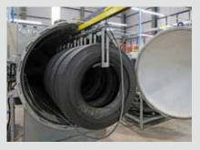
Our heat-cured tire repairs are ideal for use in retread facilities where casings are cured using large heat chambers.
