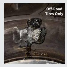
In off-road tires, multiple Permacure repairs can be bonded together to fill larger injuries
