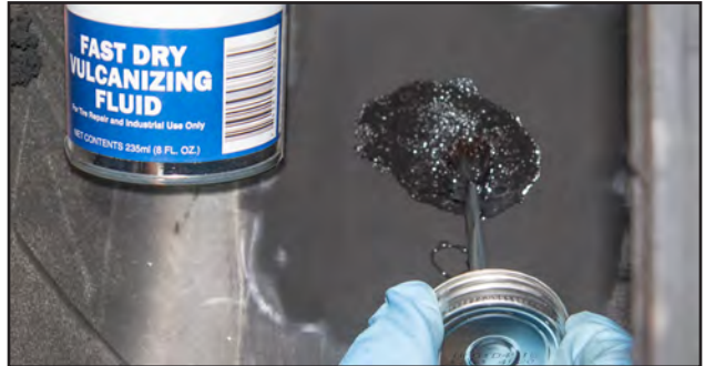
13. Apply a thin, even coat of MOR Chemical Vulcanizing Fluid (760MOR) to the buffed surface. Allow 3-5 minutes drying time. Additional drying time may be required in adverse weather conditions.
