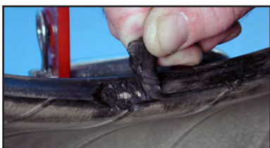
7. Deformed bead, exposed fabric or steel
