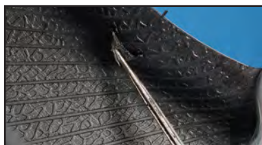
10. Tire damage from impacts
