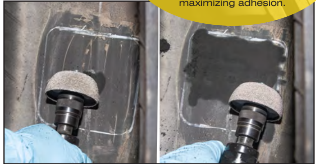
11. Using a low speed buffer (maximum 5,000 rpm) and an appropriate inner liner buffing wheel, buff the stem flush to the inner liner. Buff the entire outlined area on the inner liner to a #1 or #2 texture.
