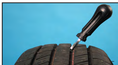
8. If injury angle exceeds 25 degrees, a 2-piece repair must be used.
