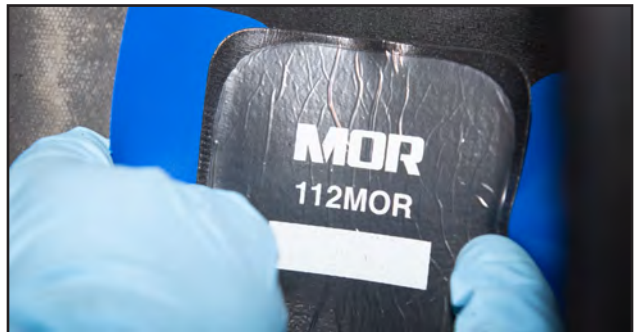
15. Relax the beads of the tire. Center the repair unit over the filled injury. Press down the center of the repair unit with your thumb.
