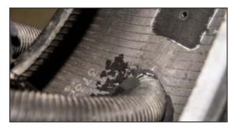
**12.** Vacuum all buffing dust from the tire. Avoid touching the buffed surface with the vacuum as this could lead to contamination.
