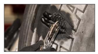
**26.** Finish filling the skive area to a level 1/8" (3 mm) above the tire's outer surface and stitch. The tire is now ready for cure.
