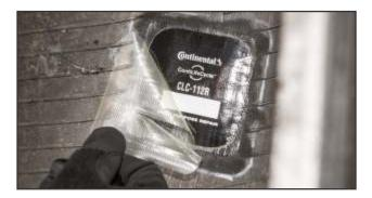
**19.** Remove the clear Mylar from the top of the repair unit by lifting from the edge of the repair and inspect the repair unit for trapped air. If trapped air is found, stitch the repair unit again. Extra attention should be paid to the repair unit edges to ensure they are thoroughly stitched.
