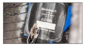
**17.** Press down the center of the repair unit. Begin stitching from the center outward. Stitch out to the folded poly.
