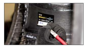
**23.** Mark the date, repair technician initials (optional), and retread plant DOT code onto the repair unit. Use a dark ink pen or marker.
