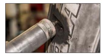
**24.** All injuries should be filled with a rubber that is approved for use without black retread cement. It is critical to apply one layer of rope rubber to the skive area due to the lack of black cement.
