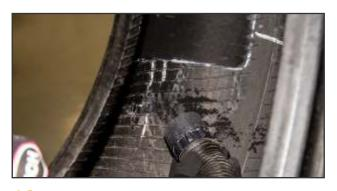
**16.** Vacuum all buffing dust from the tire. Do not touch the buffed surface with the vacuum, as this could lead to contamination. Use of an air hose to remove dust is not recommended as it will lead to contamination of the repair area.
