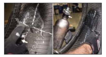
**3.** Place the tire so the repair area is in a 5 or 7 o'clock position to allow the buffing dust to fall to the bottom of the tire. Where permitted, the area can be cleaned by using CLC-704 Liquid Rubber Buff, to prevent contamination of tools. Use a scraper tool to remove contaminants. Repeat this process 2 or 3 times until all contaminants have been removed from the repair area.
