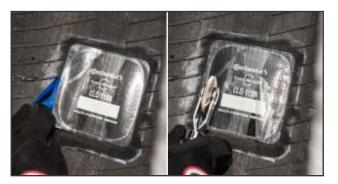
**18.** Remove the remaining poly from the repair unit and continue stitching using firm pressure. Stitch in both directions to eliminate any trapped air.
