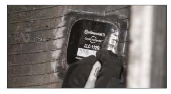
**20.** Mark the date, repair technician initials (optional), and retread plant DOT code onto the repair unit. Use a dark ink pen or marker. The tire is now ready for cure. The tire can be cured the same day or the following day.
