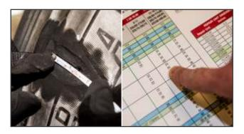
**10.** Measure the width and length of the injury at the widest opening of exposed ply to determine the section repair unit to be used. Refer to the radial repair chart for proper repair unit selection.
