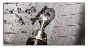
**5.** Using a small ball rasp, remove a small area of the inner liner around the injury to inspect the casing. If splits in the rubber and/or loose cables are detected, the damage must be removed. This can be accomplished by using a larger carbide cutter. If the damage exceeds ½" (10mm), the injury must be processed as a section repair.
