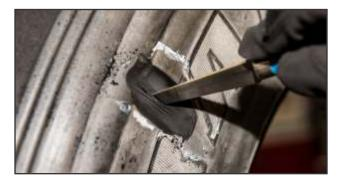
**5.** Separate damaged cables by cutting as close as possible to the damage with a sharp knife.
