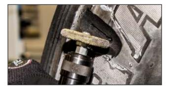
**9.** Buff the rubber above the body ply using a low RPM buffer and a medium grit rasp or encapsulated brush. Buff to a #2 or #3 buffed texture.
