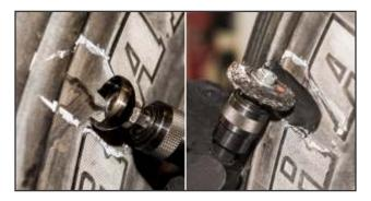
**4.** Remove all loose or damaged rubber using a knife or rotary gouge on a low RPM tool (5,000 RPM max) without damaging steel body cables. Then expose damaged cables with an encapsulated brush.
