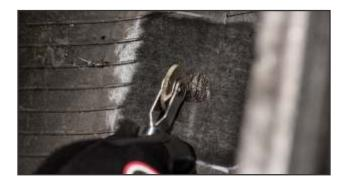
**14.** When a non-reinforced repair unit is being applied, the hole must be slightly overfilled with extruder rope on the liner side to reduce the appearance of dimples that appear after curing. Stitch the rope rubber firmly in place on the inside of the tire.
