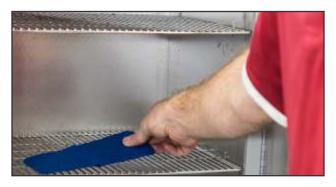
**12.** Repair units can be installed with or without floater gum. In order to achieve proper green tack, the repair unit must be heated to a temperature of between 140°F and 160°F (60°C to 72°C). 111R, 112R through CT-24R repairs should be pre-heated 5 to 7 minutes. For repairs larger than a CT-24R, the pre-heating time is 8 minutes. The use of an oven is recommended so that the repair unit can be heated thoroughly and multiple repair units may be heated.
