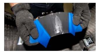
**17.** Remove the repair unit from the oven; peel back the poly half way in both directions as in any other repair method. It is also recommended that the poly be angled slightly so that one edge of the poly is outside of the edge of the repair. This makes it easier to remove the poly once the stitching process begins.
