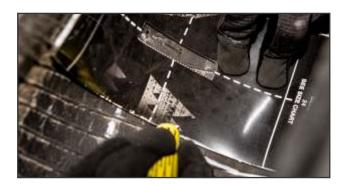
**13.** Use the appropriate repair unit template and a tire crayon to mark an area on the inner liner for buffing.
