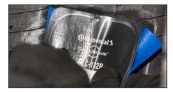
**16.** Fold the repair unit and position it, aligning the bead arrows to the tire's beads if a reinforced repair is being used. Center the repair unit over the injury. Release the repair unit and check the alignment. If the repair unit is not centered and/or straight, lift and reposition.
