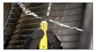
**1.** Locate and mark all damage on both the inside and outside of the tire.
