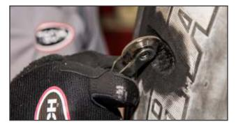
**25.** Support the repair unit on the inside of the tire. Stitch the rubber to work out any air and to assure good contact with the tire.
