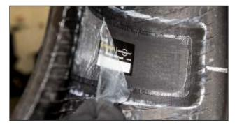
22. Remove the clear poly from the repair unit.
