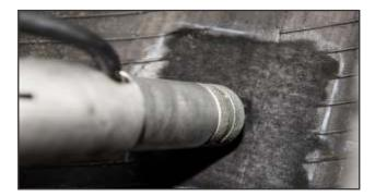
**13.** Filling the injury must be performed with rope rubber that is approved for use without cement. Preheat the extruder gun to the appropriate temperature. Place a repair unit or a piece of poly over the hole on the outside of the tire. Hold firm pressure against the tire to avoid trapping air. Fill the hole from the inside of the tire until there is about 1/8" (3mm) of rubber above the inner liner.
