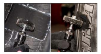
**15.** Clean the buffed areas, both on the inside and outside of the tire, using a soft wire brush on a low RPM buffer. Remove buffing dust by lightly brushing from the right side of the buffed surface to the left side. Repeat until all dust is removed.
