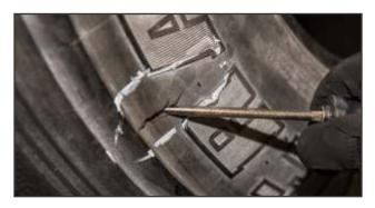
2. Using a probe, determine the size and angle of the injury while checking for rust and/or separation.
