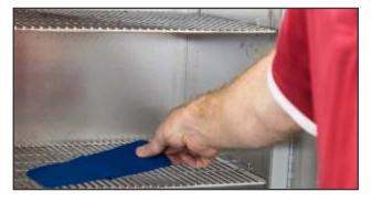
**8.** Select the correct repair unit to be installed. Refer to chart on page 11. In order to achieve proper green tack, the repair unit must be heated to a temperature of between 140°F and 160°F (55°C to 72°C). CLC-111R and CLC-112R repair units will need to be pre-heated for 5 to 7 minutes.
