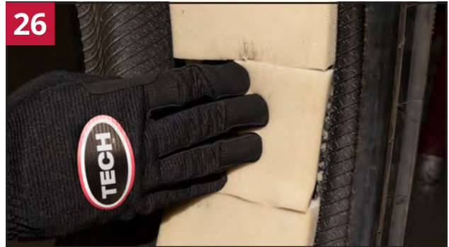
If desired, the foam can be reinstalled. If the adhesive remains tacky, simply press the removed foam back into place. If the adhesive has lost its tack, apply a layer of Security Coat #738 or Butyl Liner Repair Sealer #739 to the entire area the foam was removed from. While the material is still wet, press the foam in place and hold for 30 seconds to ensure the foam achieves proper adhesion to the tire.
