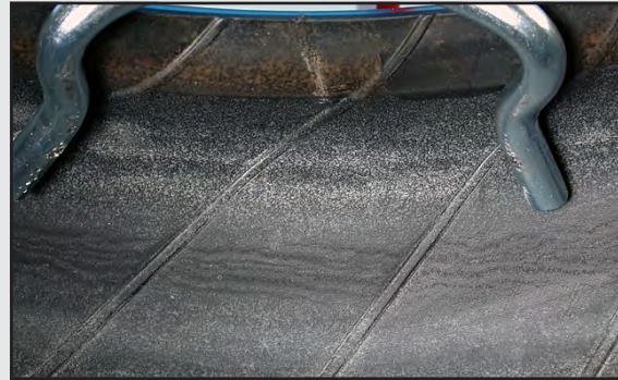
Inner Liner Cracking
